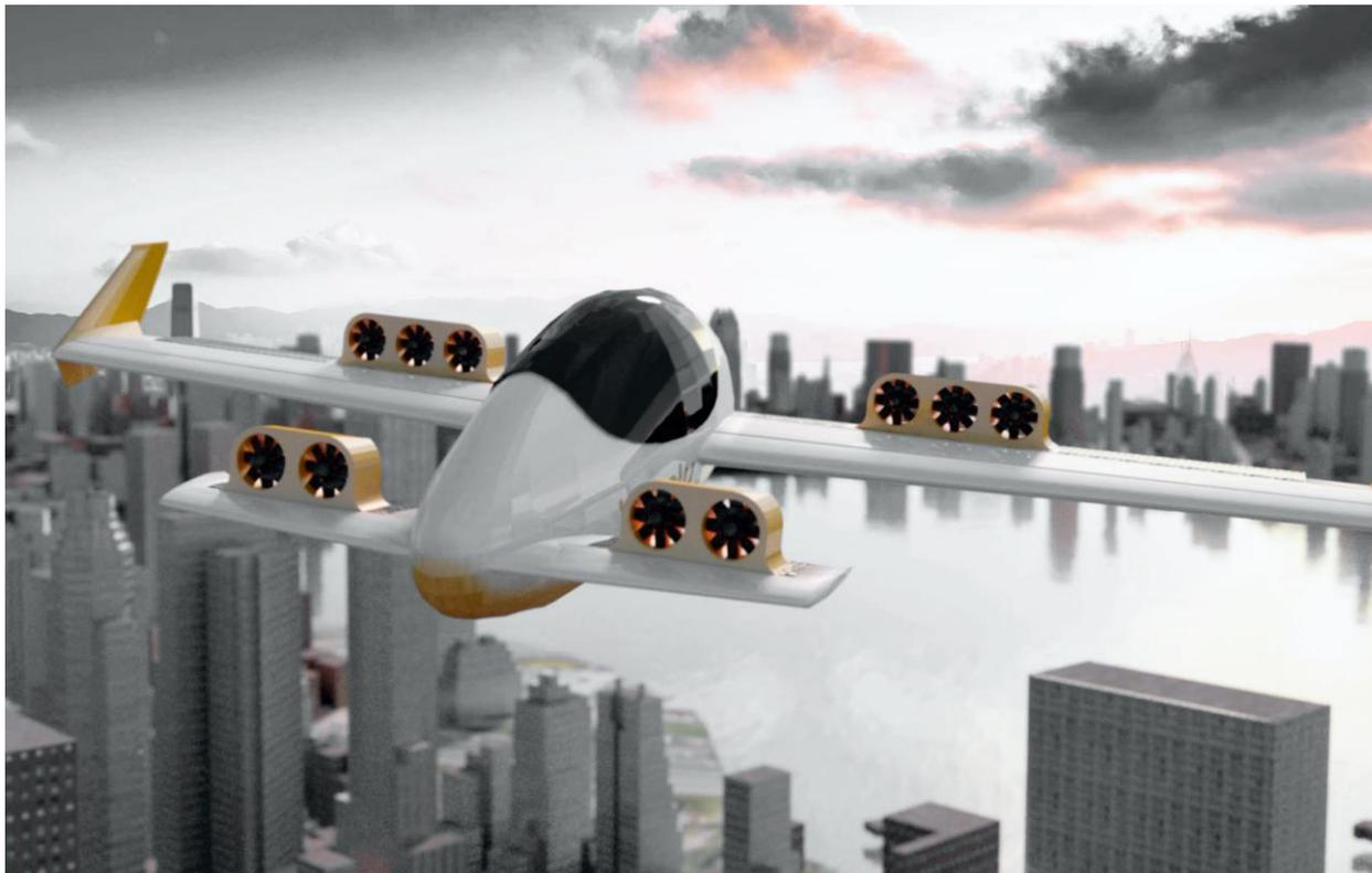
*Verpoly is a multipurpose VTOL electric aircraft designed as urban air mobility's transportation unit. Verpoly is an aircraft which uses electrical power as a driving force, making it a zero-emission vehicle. Verpoly is able to take off and land vertically, thus having a high mobility and is very suitable to be used in crowded urban cities. Verpoly also has the Poly Base feature which is a modifiable fuselage to fit various user's needs.*
