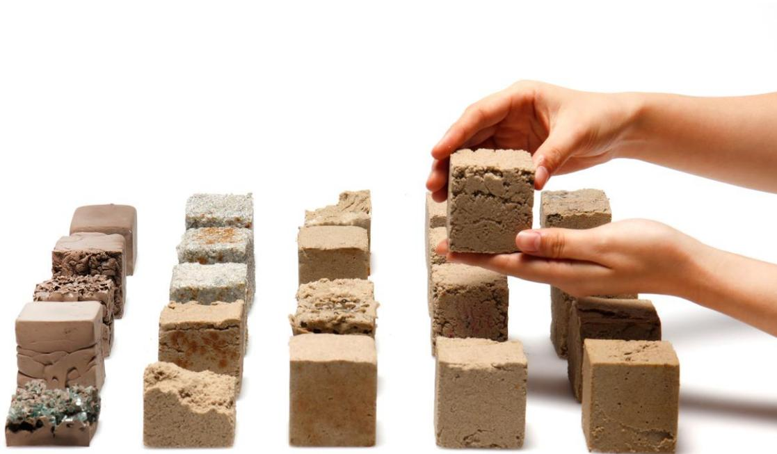
*Finite is a composite material made from desert sand. It is as strong as concrete and can be easily melted down and remoulded for multiple life-cycles or left to safely biodegrade. Finite is environmentally friendly, with less than half the carbon footprint of concrete.*
